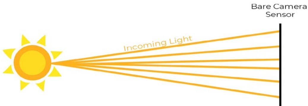
*The incoming light does not converge to a single point on the sensor. This means that everything will be out of focus in this example. Light must converge to a point to create a focus plane. That's what lenses help to do!*
